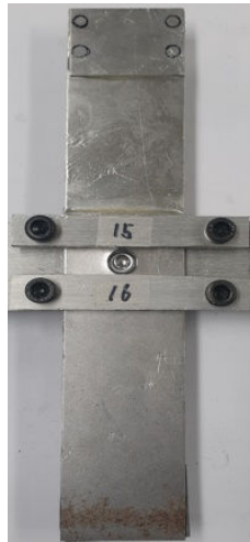
Fig. 3 Jig for fixing and adhesive hardening of the tensile-shear specimen
