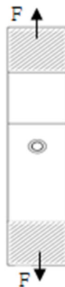
Fig. 4 Force direction of the static and fatigue test of the tensile-shear specimen
