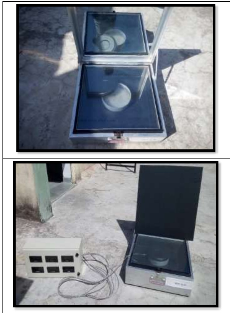
Fig. 2 Experimental Setup of Box type solar cooker with temperature sensor
