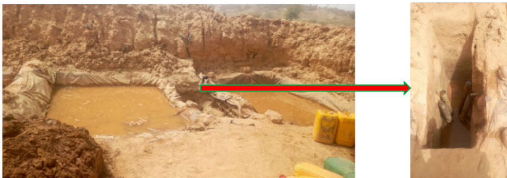
Fig. 5 Cyanidation ponds with U-shaped tubes containing the zinc chips arranged in the pool
