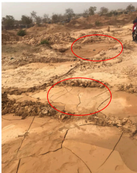
Fig. 6 Former artisanal mining holes filled with the washing sludge at Silmiougou site
