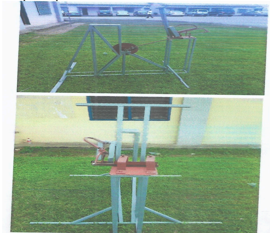
Fig. 14 Mechanical Pedal Powered Hacksaw
