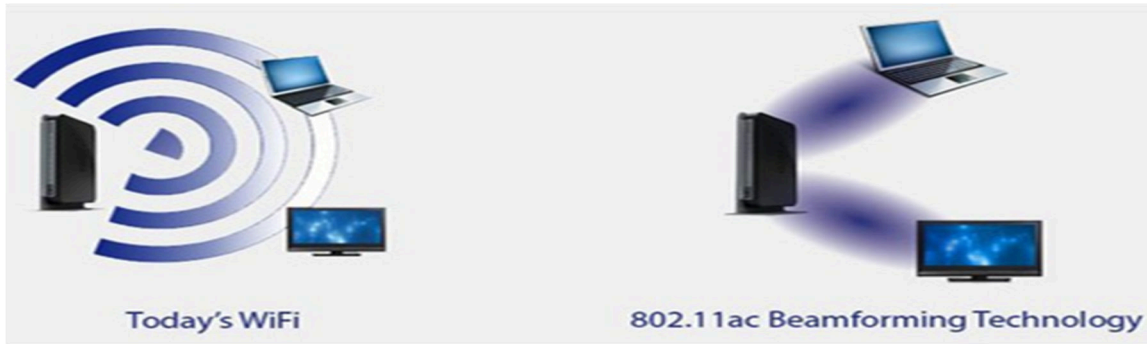
Fig. 6 Visual representation of Beam-forming technology [2]
