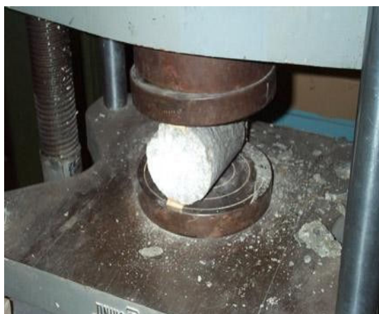
Fig. 3 Split Tensile Testing
