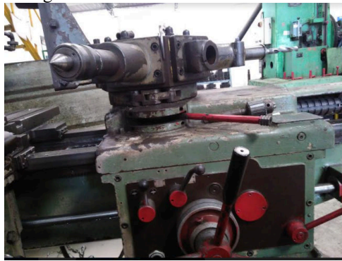
Fig.5 Original view of Indexing Turret in Industry
