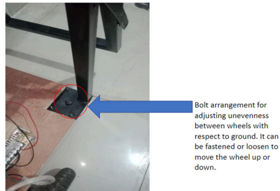
Fig. 26 Bolt for adjusting level of wheel with respect to the ground
