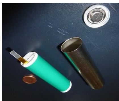
Fig. 4 Cylindrical Panasonic 18650 lithium-ion battery cell before closing.
