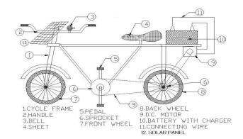
The diagram of electric bicycle determined by DC motor trim on middle shaft of bicycle & operated by battery energy shown in figure. The solar Battery riding on carriage. Solar battery generates 12V power when sun light falls on that and its stations are linked to charge controller [6].
