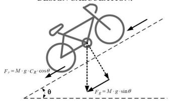
Diameter of the bicycle wheel D = 0.66m Radius r = 0.33mSpeed required s = 30km/hr Bicycle weight Wb= 20kgWeight of the rider (Approximately) Wr = 70 kg Total weight Wt = 90 kg
