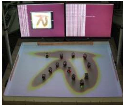
Fig. 4 Example of a coverage control algorithm executed on the Robotarium using 13 GRITSBot robots. The desired density function is projected onto the testbed arena in the shape of the letter R [4]
