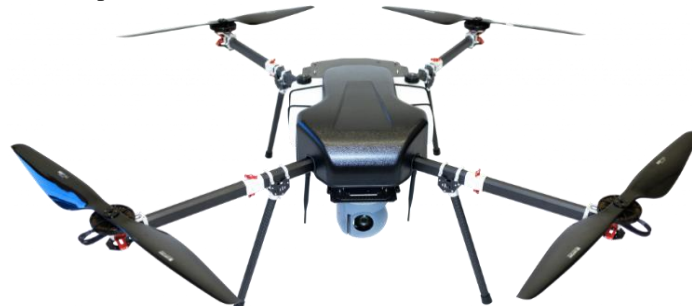
Fig. 1 The perimeter hybrid electric drone by Skyfront [5]
