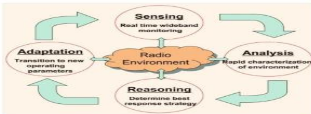
Fig. 1 Basic function of a Cognitive Radio
