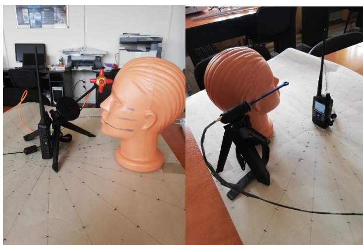
Fig. 1 The E-field probe (left) and the H-field probe (right) positioned for measurements in a plane parallel to the face
