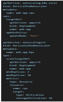
Figure 4: Example of hybrid scaling policy
