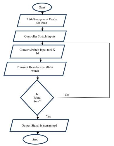
Fig. 2 System Transmitter Flowchart
