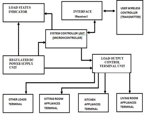
Fig. 1 System Block Diagram for Microprocessor Based Smart Home Appliance
