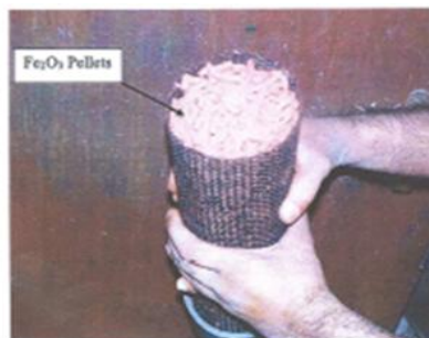
Fig. 2 Inner strainer with \text{Fe}_2\text{O}_3 Pellets
