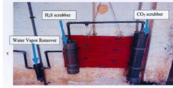
Fig. 3 Purifying Unit after assembling
