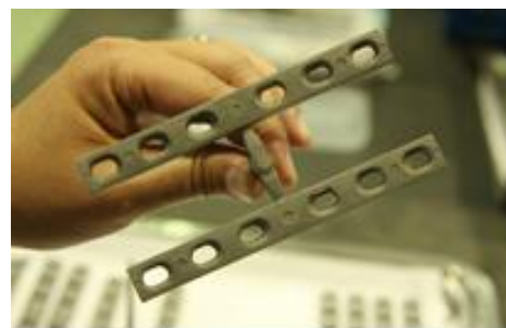
Fig. 1 Injection moulded fracture fixation plates
