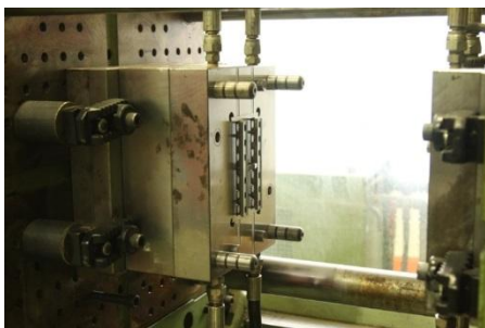
Fig. 1 Injection moulded fracture fixation plates
