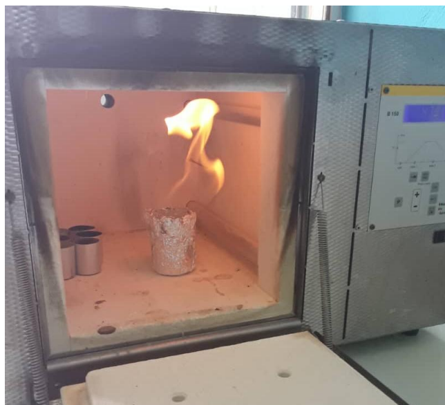
Fig. 1 Self-ignition photograph of a hydro-alcoholic gel in a muffle oven (author source)
