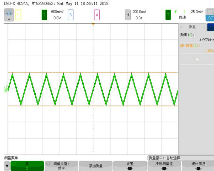
Fig. 6 Triangle Wave: u_0 = 0.51V, f = 5.0kHz
