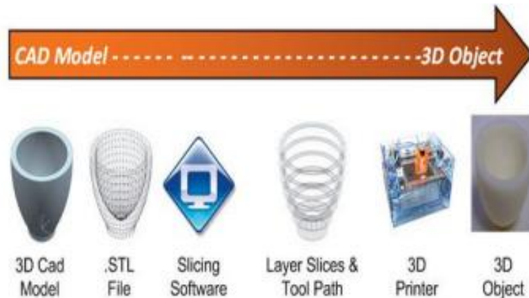
Fig. 2 Process of 3D printing (from design to printing) [10]
