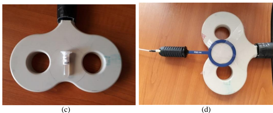
Fig. 2 a. Magstim Rapid 2 equipment with D70 Alpha coil connected for PMF exposures; b & c. Bacteria suspension samples positioned for exposures; d. H field probe positioned for the characterization of the applied magnetic stimuli
