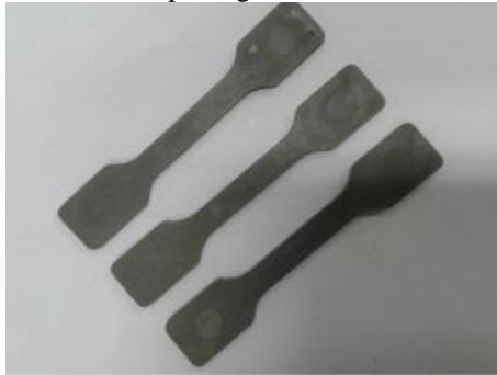
Fig. 2 Tensile specimen of the injection molded parts (green)
