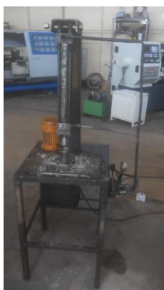
Fig. 4 Hydraulic briquetting machine
