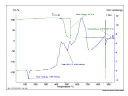
Fig. 6 TGA &DSC curve of HDPE
