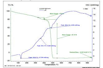
Fig. 8 TGA &DSC curve of 10 wt% treated BNHF-HDPE composite
