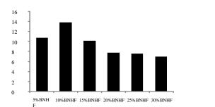
Fig. 2 Tensile strength vs wt % of untreated BNHF of untreated BNHF-HDPE composites
