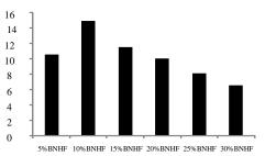
**Fig. 3** Tensile strength *vs* wt % of NaIO<sub>4</sub> treated BNHF of BNHF-HDPE composites
