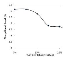
**Fig. 4** Elongation at break (%) *vs* wt % of untreated BNHF of untreated BNHF-HDPE composites
