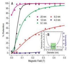
Fig. 2.2 Size Dependent Separation of Magnetite Particles following Flow through a Porous Column Exposed to a Magnetic Field
