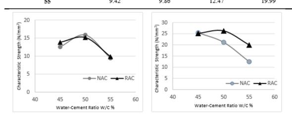
Fig. 3.3 Characteristic strength (MPa) at 7daysFig. 3.4 Characteristic strength (MPa) at 28daysTable 3.18 Weight of NAC and RAC for one cube of concrete
