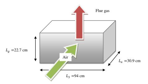
Fig. 3 Dimensions of the heat exchanger
