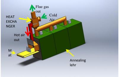
Fig. 2 Heat exchanger arrangement on the Decorating Lehr
