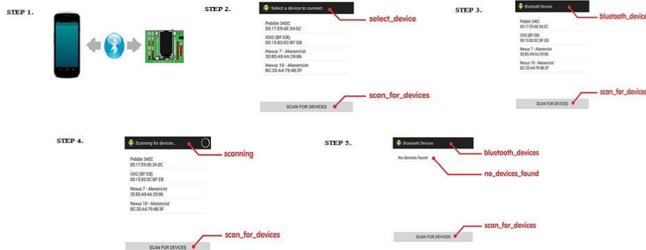
Fig. 6 Pairing process between mobile phone and Bluetooth module
