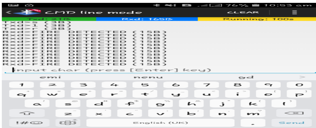
Fig. 9 When fire sensor activated
