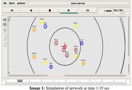
In above image the network just started and nodes are moving accordingly. The simulation time is 1.19 sec and the step of time increasing at rate of 2ms. The base station (BS) shown in red color, relay station (RS) are in blue colors and mobile users (nodes) as in yellow, orange and brown colors. The circular rings shown the active node and their respective coverage area
