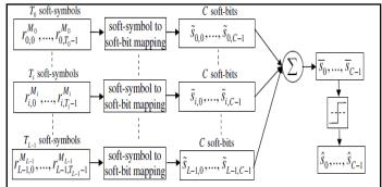
Fig. 4 SBMRC block diagram
