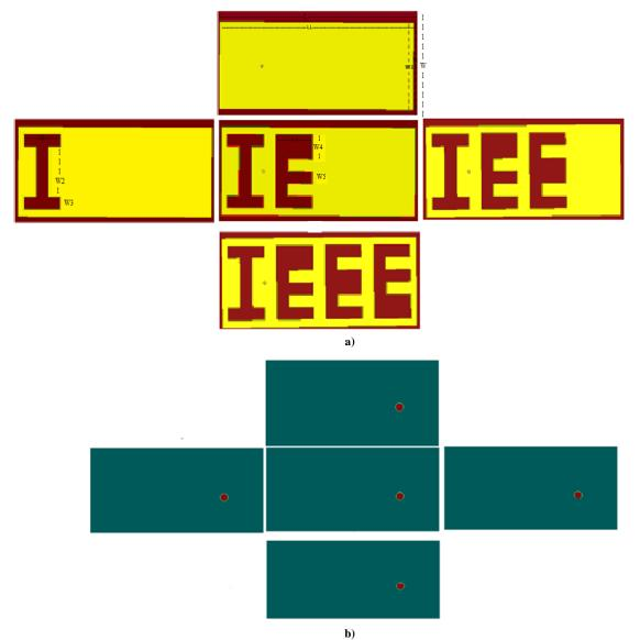
Fig.1Basic Rectangular Microstrip Patch Antenna and the subsequent slotting stages a) Top view b) Flipside view
