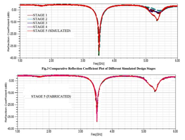
Fig.4 Reflection Coefficient Plot of Fabricated Design Stage
