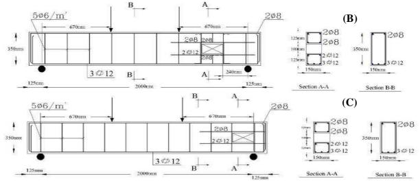
Fig. 5 Details of the Tested Specimens: (A) Beams without Opening, (B) Beams Contained Opening, (C) Beams with Different Reinforcement Details and Opening
