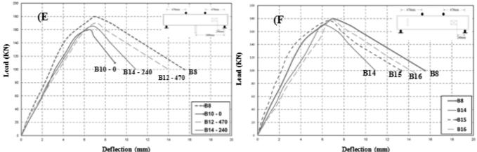
Fig. 6 Load- Mid-Span Deflection Relationship of the Tested Specimens: (A) Effect of the RCA Ratio, (B) Effect of the Shear Span with 0% Replacement of RCA, (C) Effect of the Shear Span with 50% Replacement of RCA, (D) Effect of the Location of Opening with 0% Replacement of RCA, (E) Effect of the Location of Opening with 50% Replacement of RCA, (F) Effect of the Different Reinforcement Details around Openings
