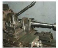
Fig.2 Pin Turning
