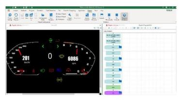
Automated Scenario Simulation: Graphical programming scenarios were created to simulate ignition cycles, speed ramps, indicator functions, and fault simulations. The use of developing reusable modular logic blocks greatly improved test simulation and promoted consistent behaviour when subjected to repeated rounds of validation cycles.
