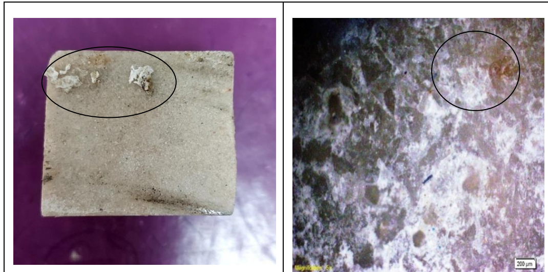
Figure 12: Surficial efflorescence associated with salt crystallization test of the studied sample and illustrated by elliptical shape (left). Stereo-photomicrograph shows slight Surficial efflorescence crystals associated with salt crystallization and marked by circle (right).
