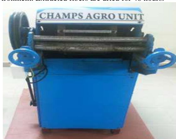
Figure 2: Fiber Extraction machine [10]
