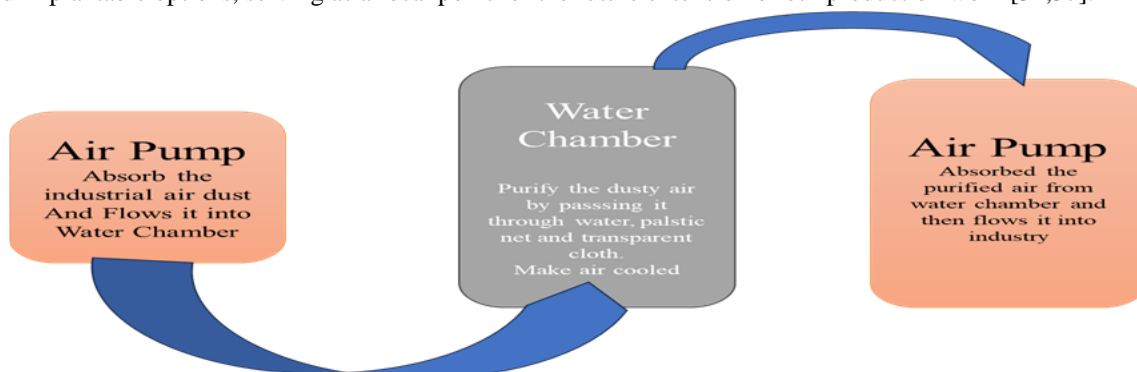
Figure 1: Flow chart of working principles for Industrial Air Dust Removing and Air-Cooling Machine
