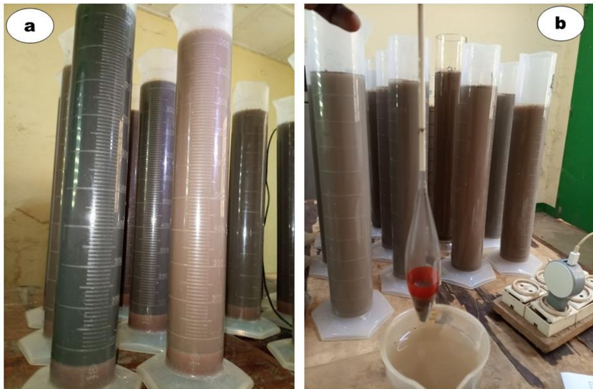
Figure 2: Particle size measurement by densimetry (a: sedimentation, b: densimetric measurement)
