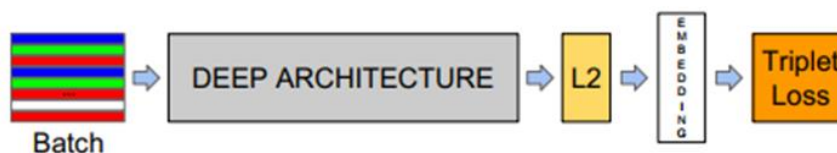
Fig. 5 Structure of the facenet network [3]
