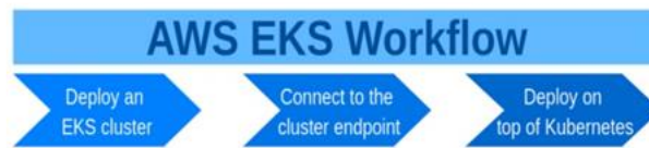
Figure 1: Schema presenting the stages of working with AWS EKS.
